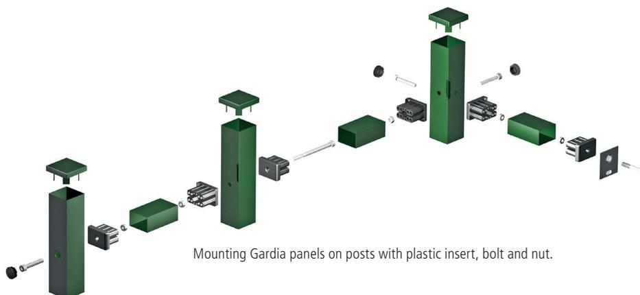
Mounting Gardia panels on posts with plastic insert, bolt and nut.
